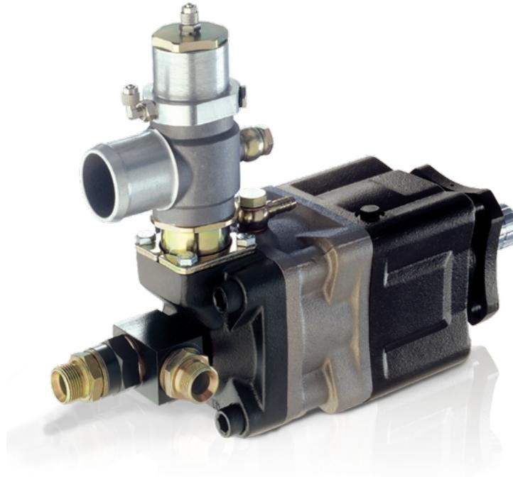
**SLPD 20/20-64/32 DIN Savtec is equipped with a shut-off valve, this makes it possible to control so that oil only feeds when required.**
