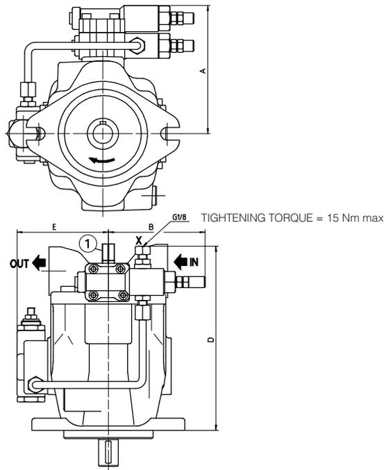
① = Regulation screw for max displacement. Adjustable range 50% to 100% of max displacement).
