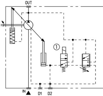
**CH Manual pressure compensator with venting**
