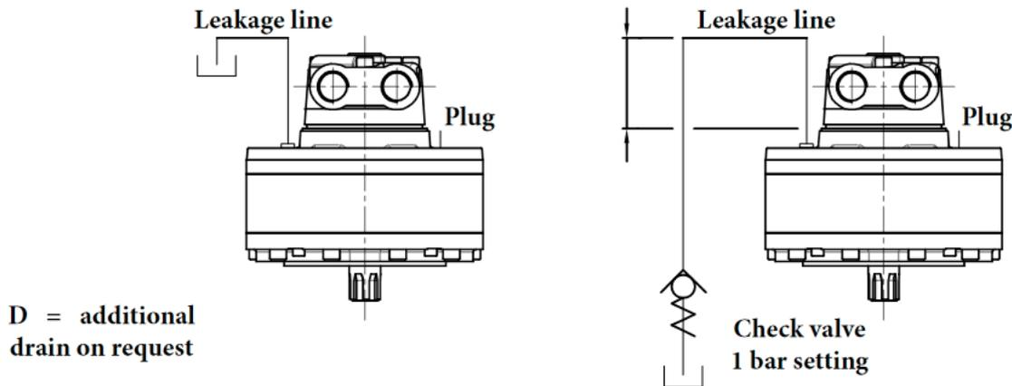
**Motor axis vertical, shaft up**
