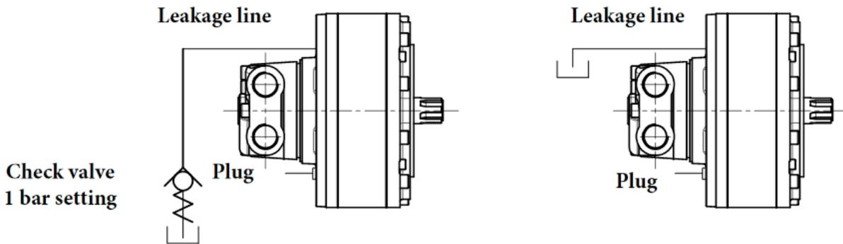
**Motor axis vertical, shaft down**
