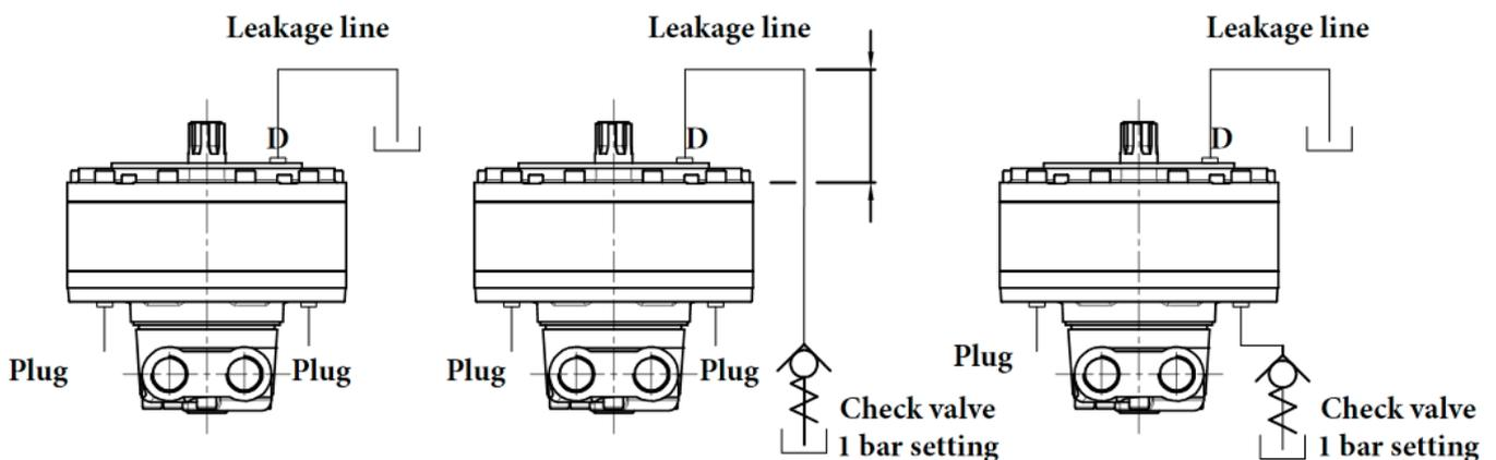
**Leakage line connection**
