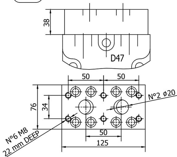
Connection block, fitting D47 distributor, for motor MR 125/160/190/200/250/300/330
