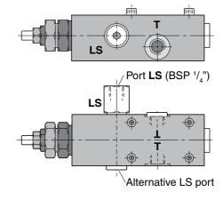
Fig. 8. VP1-095/-110/-130 control ports.
