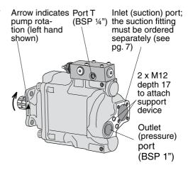
Fig. 2. VP1-095/-110/-130 main ports; left hand rotating pump.
