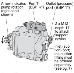
Fig. 1. VP1-095/-110/-130 main ports; right hand rotating pump.
