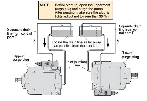
Fig. 6. Purging the VP1-095/-110/-130 (right hand pumps shown)
